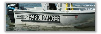
a) Visitor Assistance vessels shall be marked in such a manner to be readily identified by the public. The Corps communication mark and signature block will be mounted on the bow (front) end of the boat, and PARK
